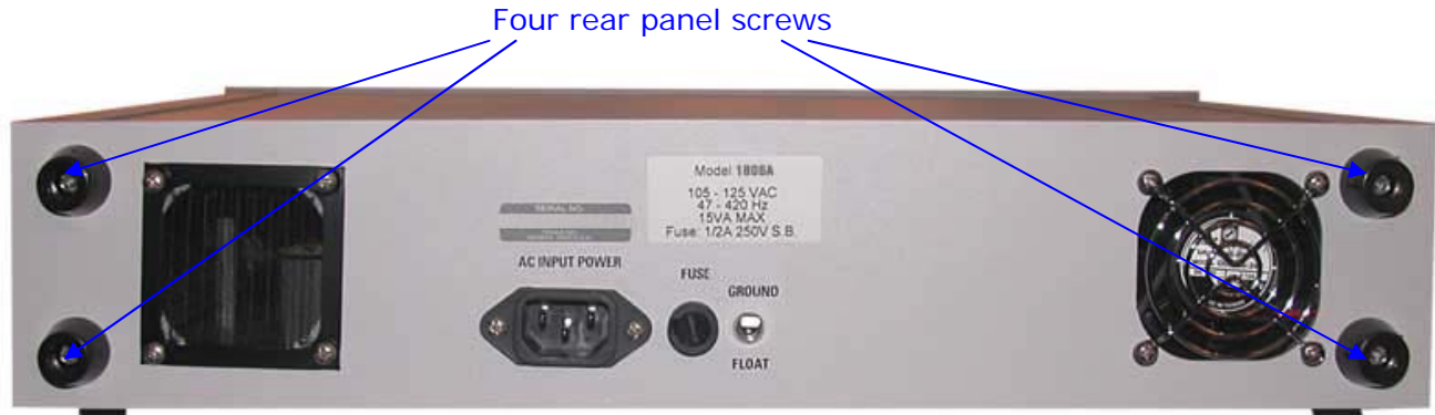
Figure 5.2 Location of Four Rear Panel Screws
